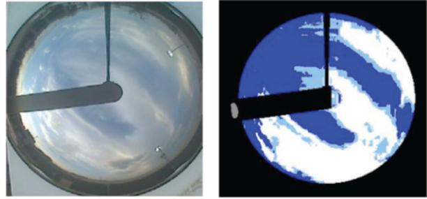
**Fig. 1** Left: example of image taken by the TSI for a cloudy day. Right: processed image using manufacturer’s image classification algorithms. White regions on lower and top right region indicate opaque clouds while thin clouds are represented by intermediate shading.
