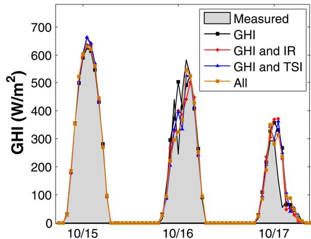
Fig. 6 GHI time series for measured and forecasted values based on  $SC_{GHI}$ ,  $SC_{IR}$ , and  $SC_{TSI}$ . The legend shows which inputs were included in the forecasting model. Night values are not included.
