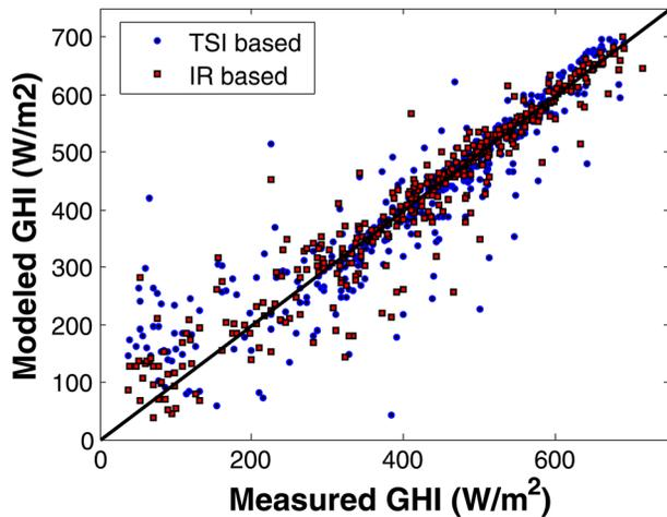
Fig. 5 Scatter plot for comparing GHI based on IR and TSI. The correlation coefficients ( $R^2$ ) for IR and TSI estimates are 0.935 and 0.923, respectively.
