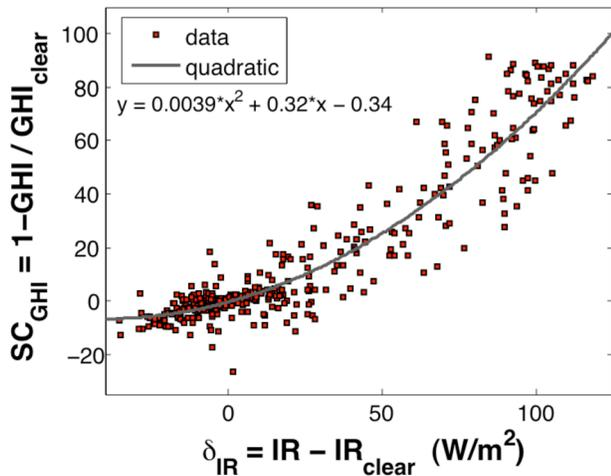
**Fig. 2** Scatter plots of  $SC_{GHI}$  versus  $\delta_{IR}$ . The line is a quadratic fit used to define  $SC_{IR}$ . The parameters of the polynomial are also shown under the legend box.
