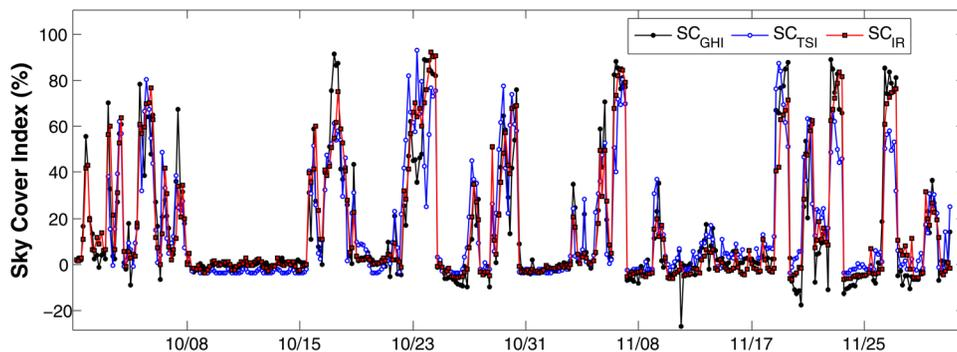
**Fig. 3** Time series of the sky cover index inferred from the TSI, IR, and GHI for October and November 2010. The night, dawn, and dusk values are excluded from the graph. The instrument maintenance day (Nov. 17) was also removed from the set shown.
