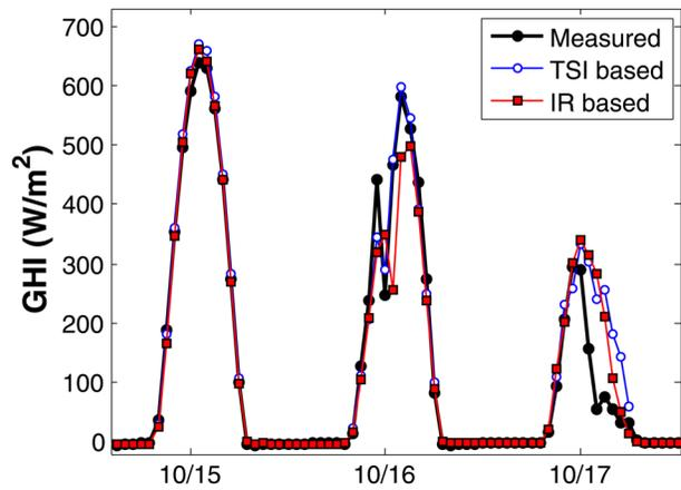
**Fig. 4** GHI time series measured and estimated based on  $SC_{IR}$  and  $SC_{TSI}$ . Night values are removed from this time-series plot.
