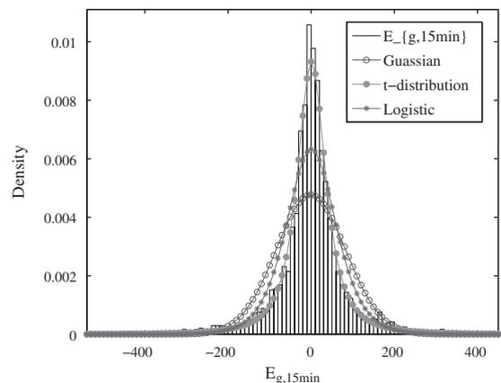
**Fig. 3.** Error distribution for 15-min load forecasting with solar penetration. The bins for the dataset are defined using Freedman–Diaconis rule. With high solar penetration the error distribution is better characterized by  $t$ -distribution.
