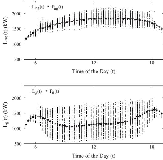
**Fig. 2.** Daily demand load profile for the UC Merced campus with no onsite power generation (top) and onsite solar power generation (bottom). The trend in the daily load profile is computed by fitting a 6th order polynomial ( $P$ ) to daily load profile over the whole year.
