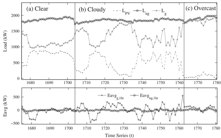
**Fig. 7.** Time-series of load and error profiles for a clear (a), cloudy (b) and overcast (c) day for 1 h forecast case. For sunny and overcast day, solar variability is the lowest and hence, the error is low too for both high and low solar penetration levels. Whereas on a cloudy day, penetration is medium but error is very high due to variability in solar power output.
