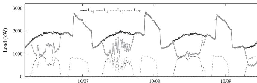
**Fig. 1.** UC Merced load profile for 06-Oct-2010 through 09-Oct-2010. The UC Merced campus has a unique load shape because the majority of the HVAC load ( $L_{cp}$ ) has been shifted to the night time using Thermal Energy Storage (TES). The total energy consumed by the campus ( $L_{ng}$ ), comprise of the energy from the solar farm and energy from electric grid, is comparatively smoother than the demand load ( $L_g$ ) that is affected by onsite solar generation.
