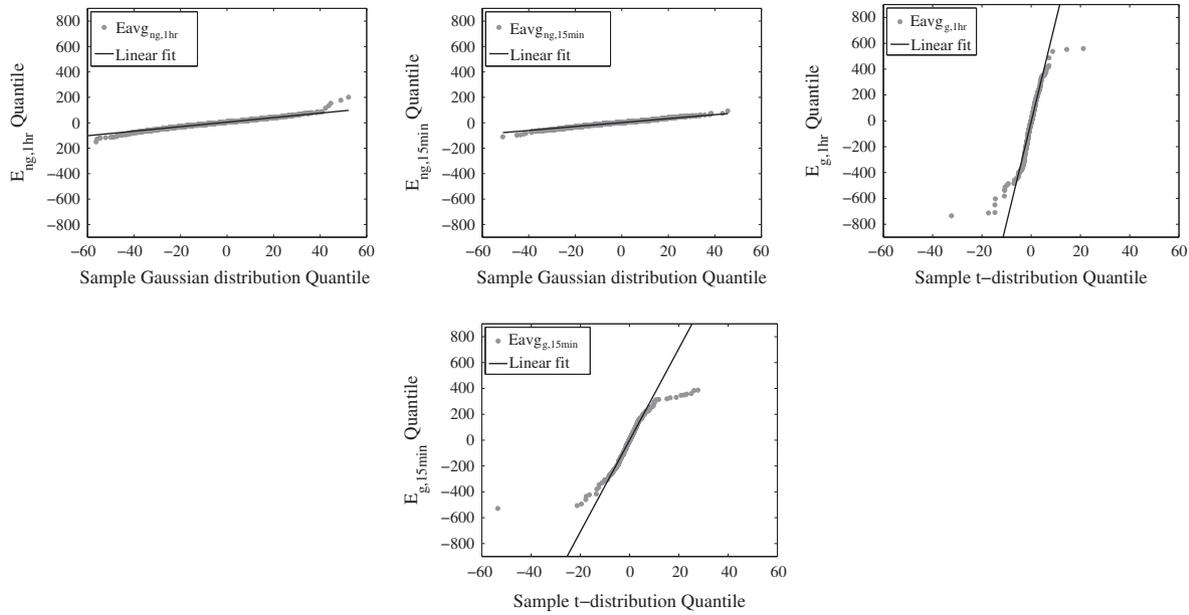
**Fig. 4.** Error distribution for 1-h and 15-min load forecasting with and without solar penetration. With no solar penetration the error distribution can be perfectly characterized by the Gaussian distribution as shown in the first and second plot. Whereas with solar penetration the error distribution can be better characterized by  $t$ -distribution. Third and fourth plot shows the sample  $t$ -distribution Q–Q plots for 1-h and 15-min cases with  $\nu=2.6$  and  $\nu=1.8$ .
