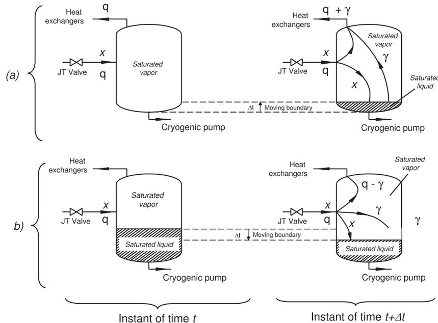
Fig. 3. Balance of mass inside the cryogenic tank, where *q* is proportion of saturated vapor, *x* the proportion of saturated liquid, and  $\gamma$  is the proportion of saturated air leaving or coming to the tank due the moving boundary of saturated liquid. Case (a) represents any simulation when liquid production is more than consumption, and case (b) when consumption is greater than liquid production.
