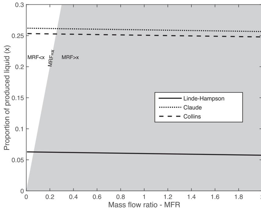
**Fig. 4.** Produced liquid ( $x$ ) versus  $MFR$  for all analyzed cycles. The white and gray areas indicate positive and negative net production of liquid, respectively.
