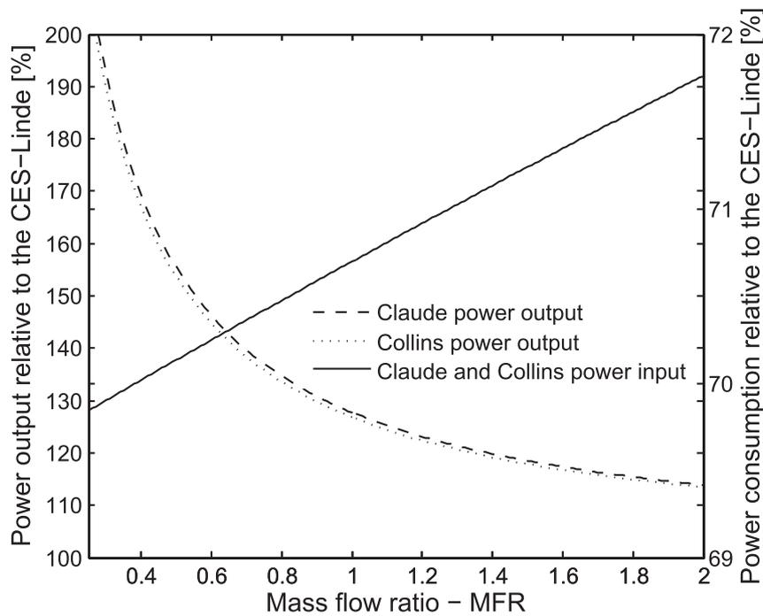
Fig. 6. Power consumption and power output as a function of MFR for the CES systems, relative to the CES-Linde-Hampson overall power output:  $\frac{\sum W_i}{(W_r)_{Linde}} \times 100$ .
