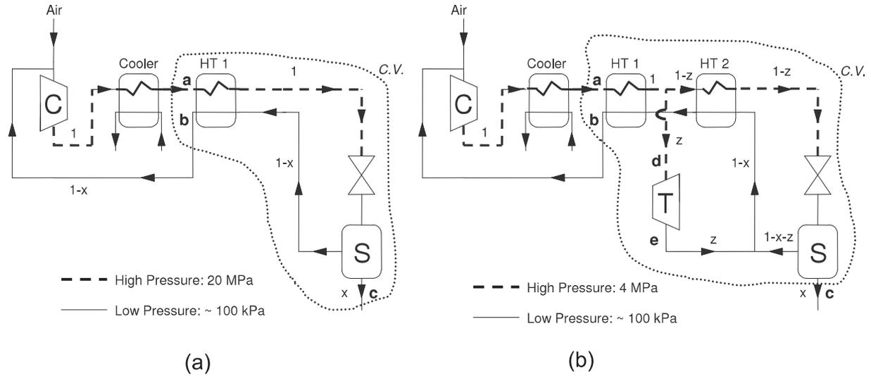
Fig. 1. (a) Schematic view of Linde–Hampson and (b) Claude liquefaction system; (C = compressor, T = turbine, HT = heat exchanger, S = storage tank).
