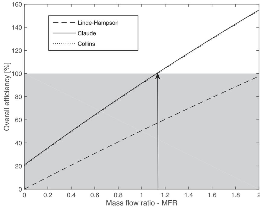
Fig. 5. Overall efficiency versus MFR for all combinations of CES analyzed.
